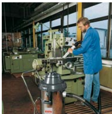
MULTISOG clean-up a boring machine
