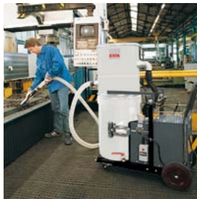
Removal of brass chips and coolants at a CNC milling station
