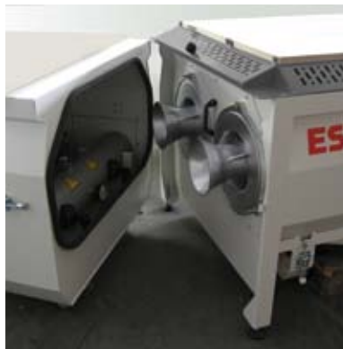
Detachable fan unit for easy access to the cartridge filter
