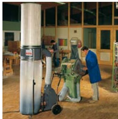
Mobile extraction unit with cartridge filter
